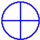
Current flowing into the conductor
